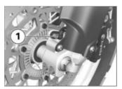
• Remove screw **1** and remove the ABS sensor from its bore.
