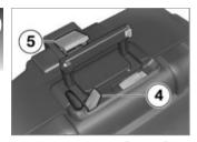
Fully open latching flap 5, if necessary pulling up red release lever 4.
