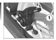
Visually inspect the brake pads to ascertain their thickness. Viewing direction: from the rear toward brake caliper 1.
