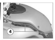
Manoeuvre the centre trim panel into position. Make sure that all three tabs 4 on left and right engage the side panels.
