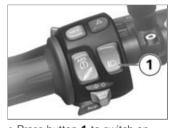
Press button 1 to switch on the auxiliary headlights.
