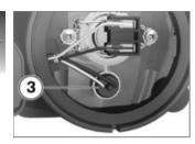
Insert socket 3 into the headlight housing.
