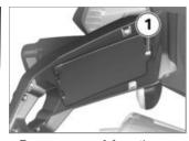
Remove screw 1 from the mudguard cover and remove the cover.
